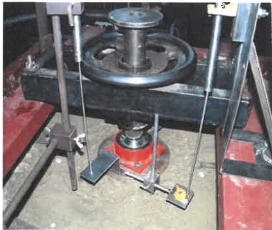
Fig. 4.4. Stand for testing static impacts on mines placed in soil [7]: - scheme: 1-hydrostatic system, 2-mounting frame, 3-pressure plate, 4-test case, 5-ground, 6-vertical displacement sensor of the mine, 7- pressure plate displacement sensor, 8-load sensor of the ground-mine system, 9-sensor of the force in mine, 10-sensor igniter's vertical displacement sensor [7]
