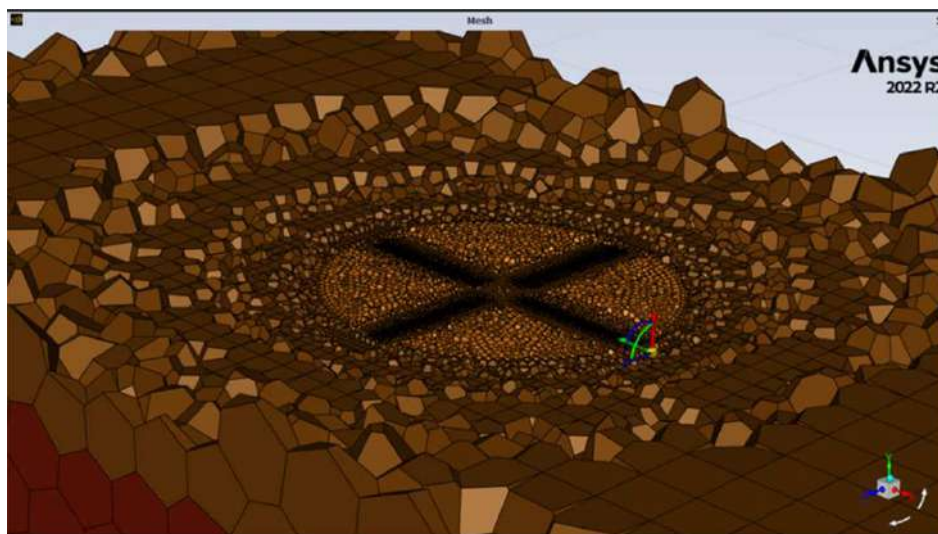
Fig. 6. Polyhexcore mesh of fluid volume elements
