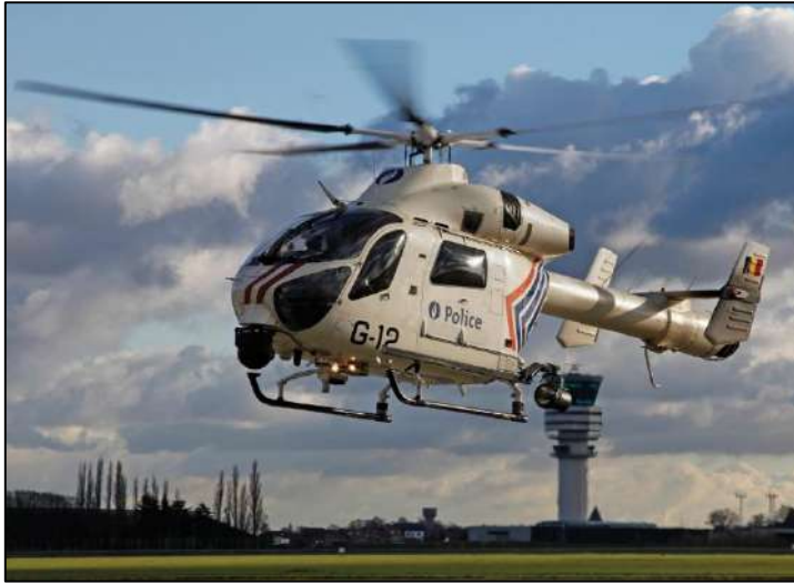
Fig. 10. MD-902 Explorer utility helicopter with NOTAR system 13
